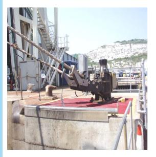
Figure 10 - Quick release hooks with capstan
